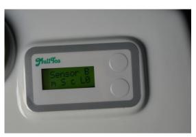
3. If there is a small letter. Lift up the toiletseat and check in display, the sensor should respond, and in display it will change from "s" to "S" to confirm. Wait 10 sec and close the seat, the letter should be small again.
