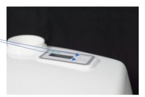
2. When you entered the service menu, move forward step by step by pushing button A. In the Sensor B window, check the letter "s". The "s" is the Seat sensor and get activated when someone visit the toilet. If there is a big "S" without seat is up go to step 7
