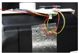
8. From step 4: Disconnect the sensor card on the mixer motor, plug in the power in the wall socket. Does the mixer start and run constant its broken and need to be replaced (in prog 2.11 the display also will show Defect motor)
