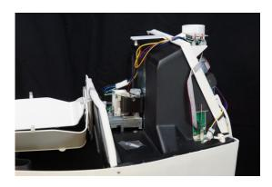
7. From step 2: Remove the socket with cable from the magnetic sensor. Check the service menu, the "S" for activated sensor should have become small "s". (If not step 9) Keep the toilet running and wait for the time schedule start the mixer. Make some kind of indicator to notice and check after 2-3 hours instead of waiting. If the mixer starts replace the seat sensor.
