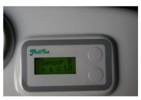
4. Move forward one step by push button A and in display you will have Output C. Check the "m", this is the mixermotor, after 20-40 sec the startpulse from the software will turn on the power to the motor and confirm by change to big letter "M". If not go to step 8
